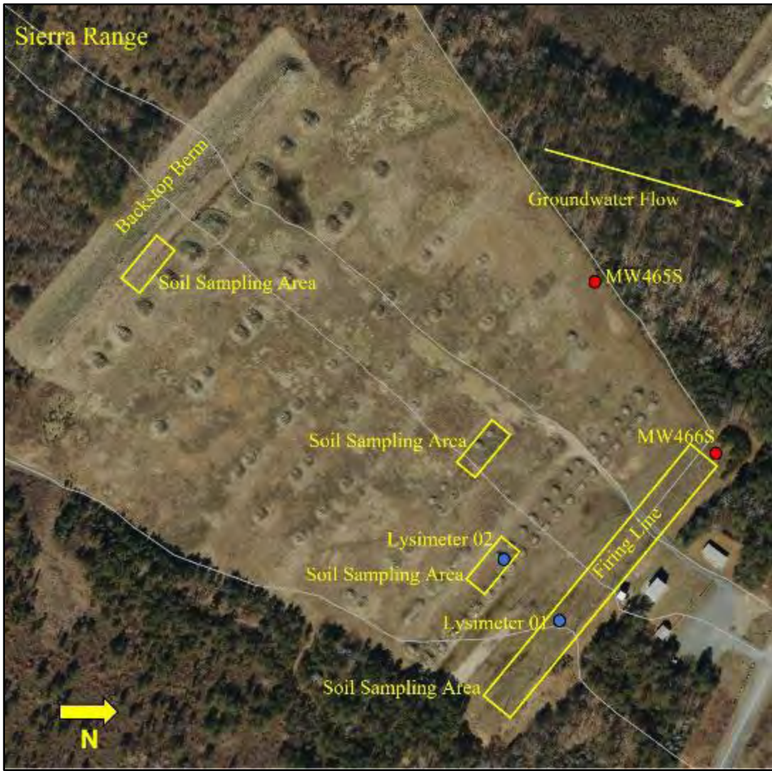
Sierra Range (EPR copper only) Sampling Areas Camp Edwards, Massachusetts MW=Monitoring Well
