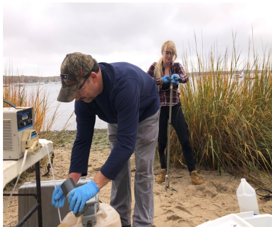
Shallow groundwater sampling near Hen Cove in Pocasset for PFOS and PFOA. The source is the past use of fire-fighting foam at the Otis Rotary on Route 28 in Bourne at the entrance to JBCC on Connery Avenue.
