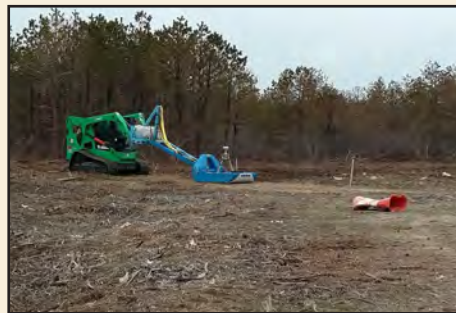
The Metal Mapper is used to discriminate between buried unexploded ordnance items and other non-hazardous metallic objects in the Central Impact Area.
